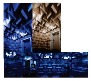
Guillemot Corporation has a professional anechoic chamber which it uses to develop its range of DJ speakers, DJ headphones and gaming headsets. The chamber's walls are covered with dihedrons made from absorbent material for measuring sound waves without any of the disruption linked to reflections, thus recreating "free field" conditions.
